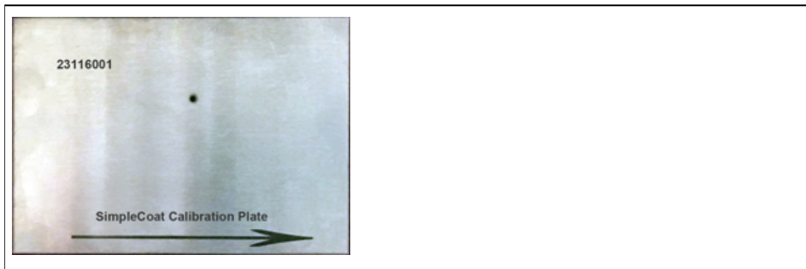
Figure 2-2. Calibration plate (PN 23116001)
