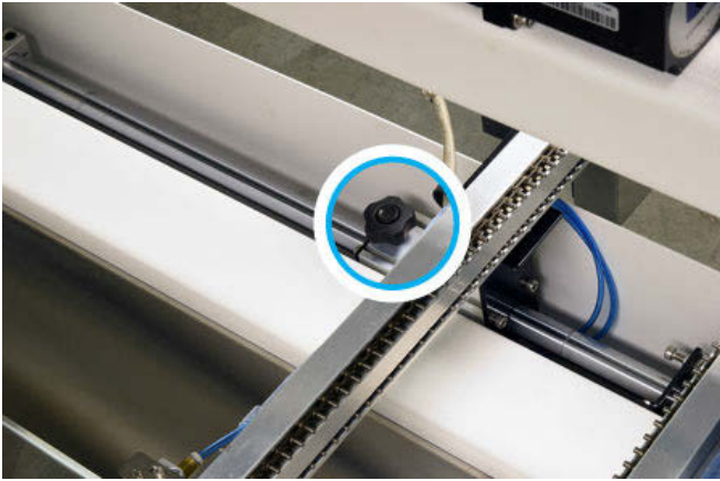
Figure 5-1. One of two conveyor locks.
