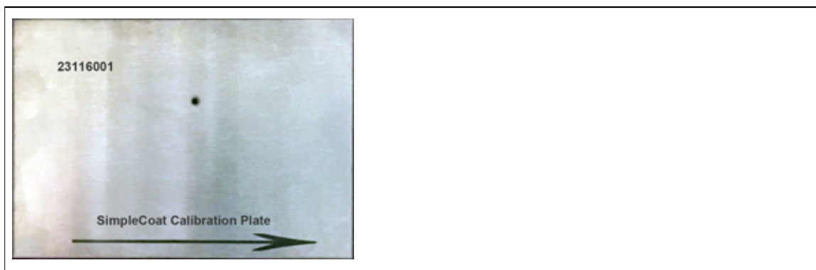
Figure 5-2. Calibration plate (PN 23116001)
