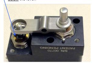
The bore in the lever faces up toward the lever/shutoff spring.
